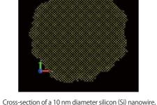
revealing modeling of the atomic-scale irregularities in the lateral surface produced during the wire formation process. In all, electron state calculations were conducted for 14 336 atoms
