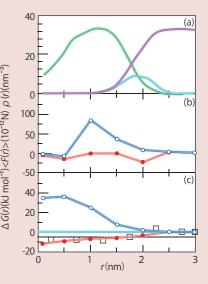
(a) Number density of the hydrophobic (----) and hydrophilic (---) of the SDS micelle and the water molecules (----). (b) Mean force and (c) free energy profile of the methane (●) and water  $(\bigcirc)$  molecules. — and  $\Box$  represent our previous work and calculation data of Matubayasi et al., respectively.
