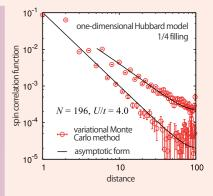
Spin correlation function of the one-dimensional Hubbard model. The numerical data are in excellent agreement with theoretical curves for Tomonaga-Luttinger liquid, which has large quantum fluctuations specific to one-dimensional systems.
