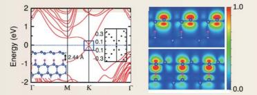
Band structure of a silicon monolayer (silicene) with a honeycomb structure and density distribution of orbits near the Fermi level. The RSDFT calculations indicated that hydrotreating of the Si (111) surface resulted in the formation of a stable silicene film, and Dirac cones were produced near the Fermi level.
