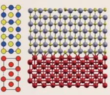
Model of compound / iron coherent interface (left) and partially coherent interface (right). Example of NbC (100) / Fe(100) interface. (Prepared by Hideaki Sawada of Nippon Steel & Sumitomo Metal Corporation)
