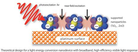
characteristics. Clear couplings of electrons and electromagnetic fields are produced through near-field light interaction
