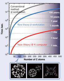
New theory and massively parallel implementation enable us highly accurate calculation of organic conductors.
