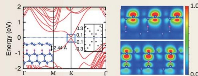
Band structure of a silicon monolayer (silicene) with a honeycomb structure and density distribution of orbitals near the Fermi level. The RSDFT calculations indicated that hydrotreating of the Si (111) surface resulted in the formation of a stable silicene film, and Dirac cones were produced near the Fermi level.
