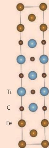
Fe(100)/TiC(100) coherent interface model (5-layer/5-layer supercell)
