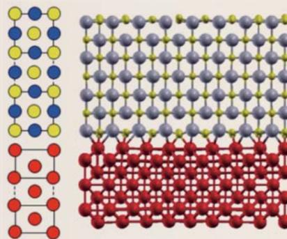
Model of compound / iron coherent interface (left) and partially coherent interface (right). Example of NbC (100) / Fe(100) interface. (Prepared by Hideaki Sawada of Nippon Steel & Sumitomo Metal Corporation)
