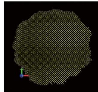
Cross-section of a 10 nm diameter silicon (Si) nanowire, revealing modeling of the atomic-scale irregularities in the lateral surface produced during the wire formation process. In all, electron state calculations were conducted for 14,336 atoms.
