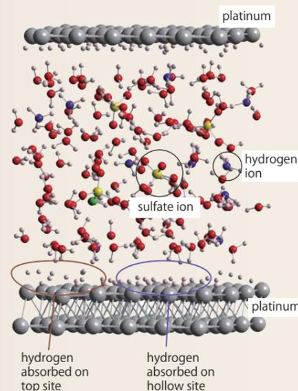
Snapshot of a hydrogen decomposition reaction simulation at a platinum-electrode interface. The ESM method realized the simulation in an environment in which voltage was applied, making it possible for the first time to reproduce the hydrogen decomposition reaction in a real matter.
