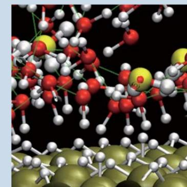
Electrode interface model of  $H_2O/Pt(111)$ . Pt (111) -  $3 \times 2\sqrt{3}$  unit cell includes 32  $H_2O$  molecules. A proton is hydrated.
