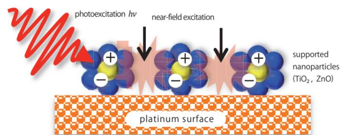
Theoretical design for a light energy conversion nanodevice with broadband, high-efficiency visible light response characteristics. Clear couplings of electrons and electromagnetic fields are produced through near-field light interaction occurring in orderly rows of nanoparticles placed on the platinum (Pt) surface.
