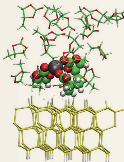
Snapshot from MD simulation of the electrode/electrolyte interface of a lithium-ion battery: desolvation of the lithium ion (in black) from propylene carbonate in the vicinity of the electrode.
